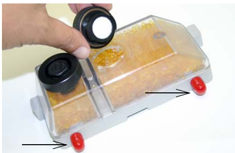
Figure 4-5 Opening the desiccant cartridge chambers
