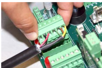
Figure 3-6 Attach wire terminal strip to connector case socket
