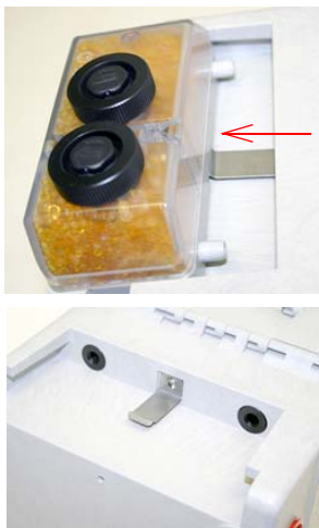
Figure 4-4 Removing the external desiccant cartridge
