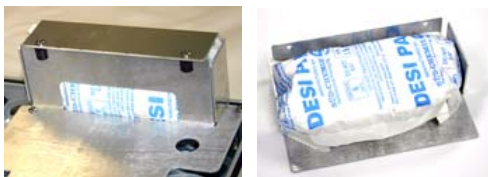
Figure 4-1 Removing the internal desiccant bag
