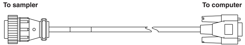
Figure 4-1 5800 Sampler to RS-232 serial communication cable (DB9-pin version shown)
